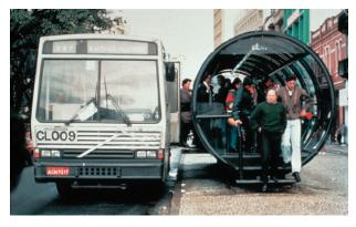
platform. The tube stations serve the dual purpose of providing passengers with shelter from the elements, and facilitating the efficient simultaneous loading and unloading of passengers, including wheelchairs. A typical dwell time of only 15 to 19 seconds is the result of fare payment prior to boarding the bus and same-level boarding from the platform to the bus.
