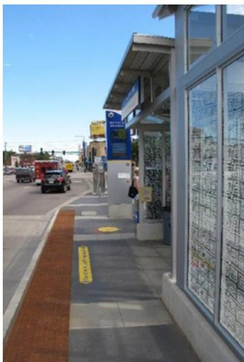
*Improving both old and new bus stop designs is important. Stops should be highly visible, and lines and directions should be clearly marked. Comfort, safety, and accessibility can be provided through seating, shelter, cameras, and wide access routes. (Photo: Snelling and University A-Line bus stop)*
