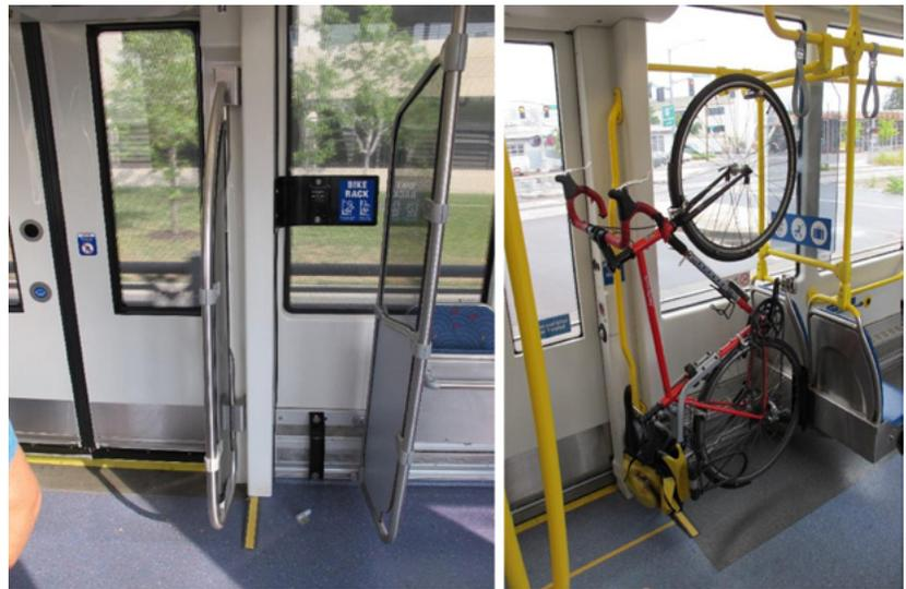
**Figure 8-7** Bicycle storage on light rail in Minneapolis and Portland, consisting of upright hanging cleats adjacent to door
