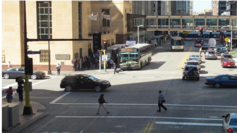
Near-side bus stops have drawbacks as well. If a near-side bus stop is located in a travel lane, it prohibits automobiles behind the bus from crossing the intersection or turning right. Near-side bus stops also limit the effectiveness of traffic signal prioritization.
