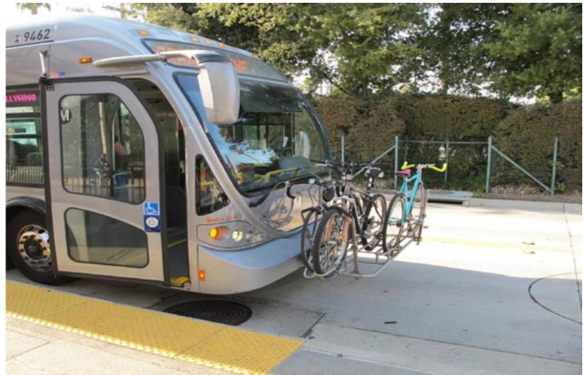
**Figure 8-6** Metro Orange Line BRT bus in Los Angeles with front-loading bicycle rack for three bicycles
