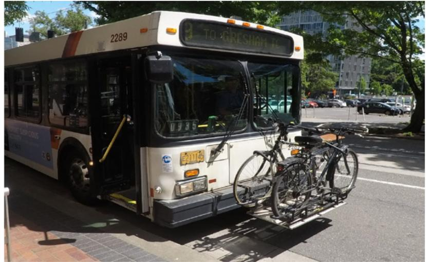
**Figure 8-5** TriMet bus in Portland with front-loading bicycle rack for two bicycles
