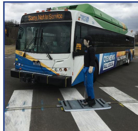
A Pierce Transit bus equipped with the AEB system being tested at the VTTI Smart Road Facility Virginia Tech Transportation Institute
