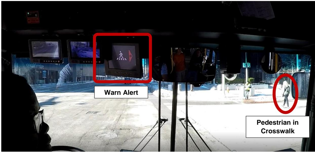
**Figure I-4. Warn Alert – Red Display for Pedestrian in Crosswalk**
