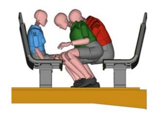
Occupant #9 was seated in a forward-facing seat without any monument directly ahead. Since this is a very singular position, the occupant started moving forward until it hit the floor ahead. For this occupant, high neck injury values as well as higher femur forces can be observed (Figure 6-23).
