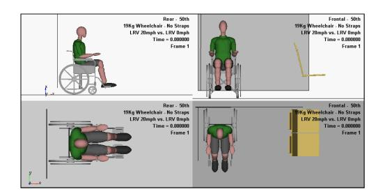
After analyzing different conditions and understanding the principal problems associated with the positioning of wheelchairs, it is possible to conclude that some type of restraint system should be used, or designed, to improve the safety for this type of occupant. Wheelchair with Straps Load Analysis
