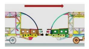
Figure 4-20 shows the kinematics of this simulation. At 185 ms after the impact, the maximum values are obtained for the neck moments. Similar conclusions as those obtained for the LRV type N were obtained. Most of the injuries occurred to the neck region due to its direct or indirect impact with the headrest.
