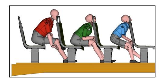
For occupants seated on facing seats (#4, #5 and #6), only occupant #6 had low injury values. Occupant #4 had a high neck extension because of the aft-facing seat. At the same time, high femur forces can be observed on occupants #4 and #6 because of the direct impact between their low extremities (Figure 6-37).
