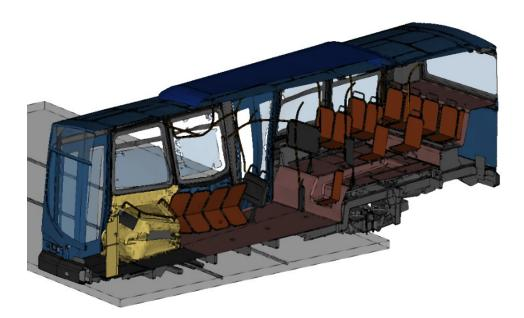
Figures 6-15 and 6-16 show the impact kinematics. Figure 6-17 shows the acceleration pulse profile of the LRV during simulation. The largest acceleration recorded is slightly above 4 g's.
