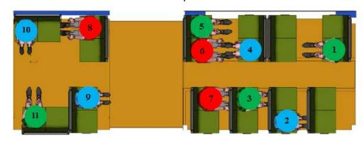
The colors used for this analysis are blue for the 5<sup>th</sup> percentile ATD, green for the 50<sup>th</sup> percentile ATD, and red for the 95<sup>th</sup> percentile ATD. Table 6-2 shows the number used for each ATD and a description of its location.
