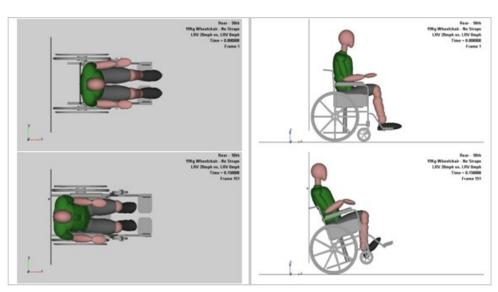
Configuration 2— Wheelchair without Straps with  $50^{th}$  Percentile ATD—Contact Moment t = 400 ms
