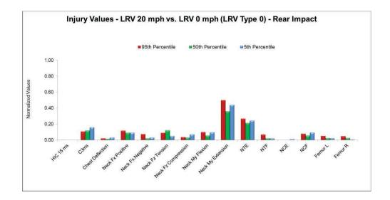
Figure 4-23 shows the kinematics of the simulation. The moment of maximum extension for the necks of the three occupants occurs around 200ms. Almost no differences are found between types N and 0. The larger values observed for the neck extension is again due to the seatback design.
