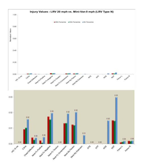
Due to the low level of energy absorption by the LRV, the injuries observed are much lower than current FMVSS 208 limits (Figure 4-9). Because no injuries were observed this crash scenario was not studied for rear impact conditions, or with aft facing seats.
