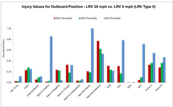
Figure 5-6 summarizes the results from the outboard and inboard configurations. As a consequence of using forward-facing seats for this configuration, similar results as the ones obtained in Section 4 were observed. The 5th percentile has very high injury values due to the headrest design. The 95th percentile has also some high results for the inboard configuration on the neck region. Finally, the 50th percentile has all the injury values analyzed between the limits.
