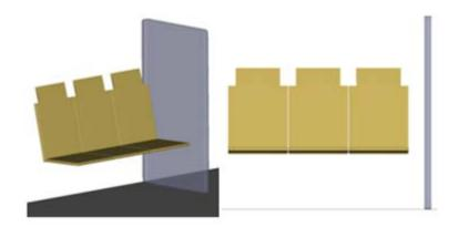
The weight of this barrier is 4 kg. This type of barrier is usually attached to the LRV at the ceiling and floor, and occasionally the outer edge is attached to the LRV
