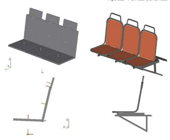
The layout survey in the "Survey of LRV Specific Interiors" shows the different configurations. One of these configurations is the lateral-facing seat with a monument barrier. This barrier can be found on either side of the lateral-facing seat. With the intention of representing this configuration, a generic multibody model of a common barrier was created (Figure B-3).
