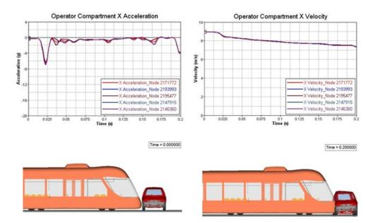
The acceleration pulse obtained through the FE model above (Figure 4-8) was used in the multi-body model shown below in Figure 4-6 to evaluate possible injuries. All injuries are normalized with FMVSS 208 limits so they can be shown in the same bar chart. Figure 4-8 shows the kinematic of the simulation at 0 ms and 250 ms. Because of the low pulse, no contact between occupants and seats was observed.
