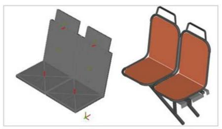
The total weight of the double seat is 32 kg and is distributed as follows:
