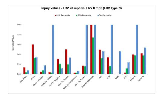
Figure 4-16 shows the injury values normalized according to the FMVSS 208 limits. Once more, the 5<sup>th</sup> percentile incurred the largest injuries. The 95<sup>th</sup> percentile also has some injury values above current limits. The 50<sup>th</sup> percentile values were below the acceptable limits; however, values for the neck region were relatively large.
