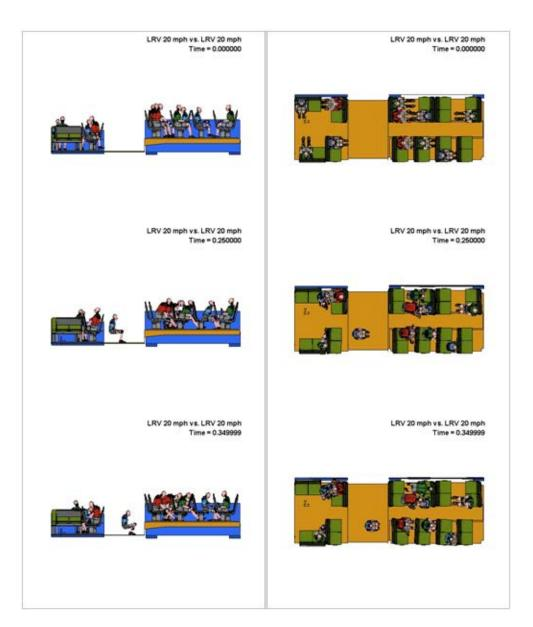
Kinematics Progression of Occupants during High-Energy, 90-Degree Impact of LRV at 20 mph and LRV at 0 mph—0 to 350 ms Impact Moment
