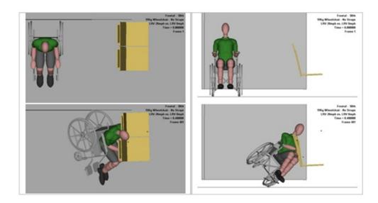
According to the injury values shown in Figure 5-78, the configuration with the wheelchair in the longitudinal direction of the LRV has very large injury values for both the head and neck regions. Due to the lack of anchor points, the wheelchair rotates, thus allowing the occupant to impact the monument. The properties used for the contact between the head and monument are the same as those used for the barrier from the lateral-facing seat study.
