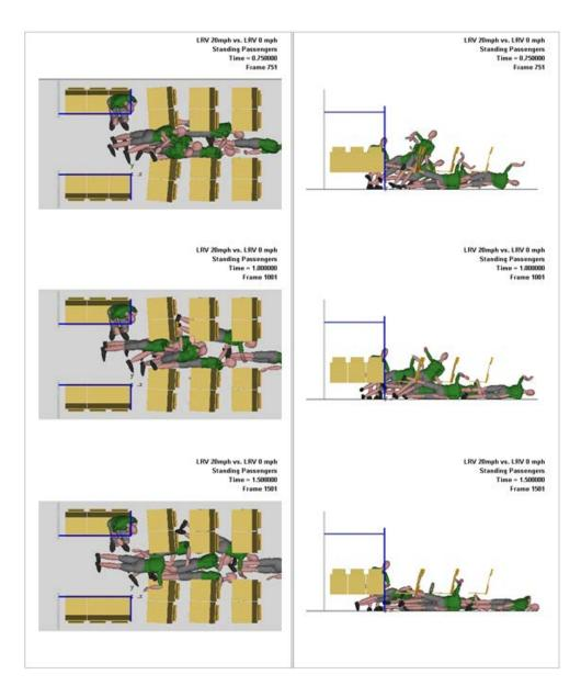
Position of Passengers Standing in Aisle between Side-Facing Seats at 750 to 1,500 ms Impact Moment
