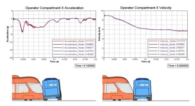
For this scenario, the acceleration pulse shape is similar to the low energy scenario. However, the average acceleration in the x-direction is approximately double that obtained for the low energy impact condition.
