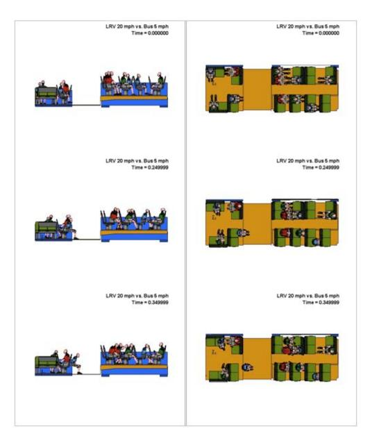
Kinematics Progression of ATD Occupants during Low-Energy, 90-Degree Impact of LRV at 20 mph and Mass Transit Bus at 5 mph—0 to 350 ms Impact Moment
