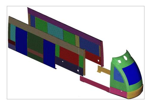
Figure 6-6 shows the finite element model for a complete car. Usually, LRVs are constructed using two main cars and a middle car where the articulation mechanisms are placed. For that reason, to complete the model, the car shown here is reflected along the X-axis and a middle cabin is created. The middle cabin is created so the length of the LRV matches the dimensions specified in the model characteristics.
