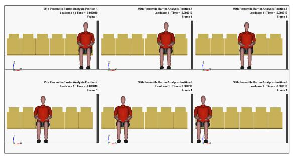
To summarize, in general, the maximum impact velocity for the ATDs appears when they are placed on the second seat. In this position, the passenger has enough time to build up the maximum velocity and, at the same time, the impact surface is very close. Thus, the worst injuries can be expected in this position. Although the maximum velocity reached by the passengers was the same when sitting in positions three to six, the impact velocity was smaller due to the friction with the seat surfaces.
