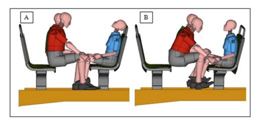
For this high-energy impact, occupant #5 impacted the facing seat in front of it. Consequently, high injury values were observed for neck extension and neck compression (Figure 6-38). Also, femur forces were higher than those obtained during the low-energy impact.
