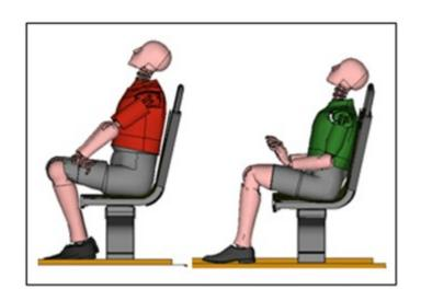
The occupants seated on the forward-facing seats (#2, #3, and #7) had different level of injuries depending on their sizes. Occupant #2, which is a 5<sup>th</sup> percentile ATD, had a very large neck extension because of the impact with the handrail. This occupant also had high chest acceleration due to this impact. Occupant #3 had the same problem with its neck extension. Nevertheless, all remaining injury values are very low. On the other hand, occupant #7 had low injury values
