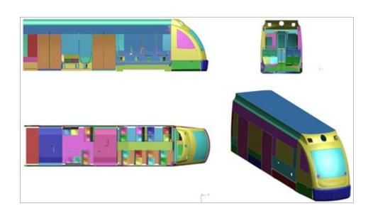
The total length for this model is 29,370 meters. It represents a Category 2 LRV with CEM components, and an empty weight of 44,769 tons. Being a Category 2 vehicle, this LRV has 70 percent of the floor at low level. Figure 6-7 shows the completed LRV model.
