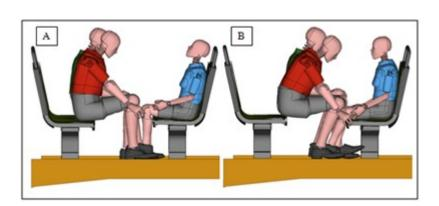
Occupant #5 suffered high femur forces because of the impact with the empty facing seat (Figure 6-22). Although all the injury values were low, higher neck injuries could be expected once the occupant impacts the front seat back.
