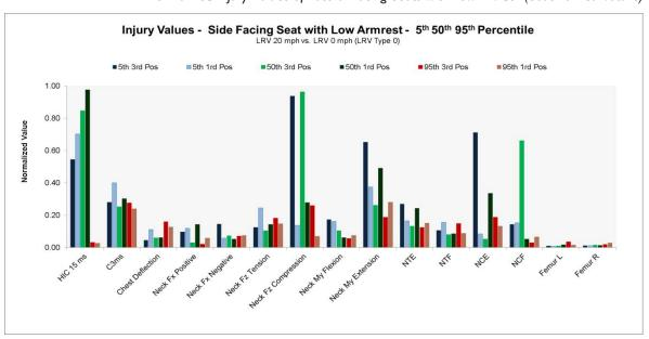
**Figure 5-62**Normalized Injury Values of Lateral-Facing Seats with No Divider (Original Results)
