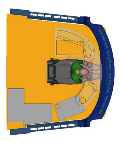
Instant of Maximum Femur Forces of Operator during High-Energy, 90-Degree Impact at 272 ms Impact Moment The kinematics progression of this high-energy impact at various impact moments is shown in Figure 6-47 and Figure 6-48.
