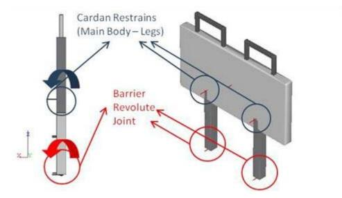
The total weight of the barrier is 21 kg (18 kg main body and 3 kg each leg). The main dimensions are as follows:
