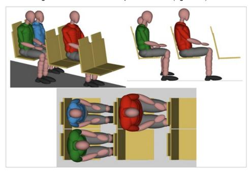
As explained above, three ATDs were used in this model. To help distinguish between ATDs, three different colors were used. These colors remain constant throughout the report. Red is used for the  $95^{th}$  percentile, green for the  $50^{th}$  percentile, and blue for the  $5^{th}$  percentile.
