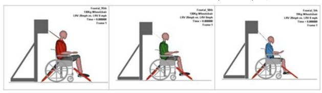
The acceleration pulse used for this analysis is the LRV type 0 traveling at 20 mph and impacting another LRV which is stationary at 0 mph. Both frontal and rear impact conditions were studied. The worst-case scenario is the rear-impact condition, due to the transfer of load between occupant and wheelchair. For the frontal-impact condition, the occupant is restrained by a three-point belt system, which reduces the amount of force transmitted to the wheelchair anchors.
