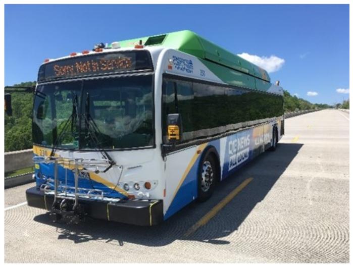
A Pierce Transit bus equipped with the AEB system being tested at the VTTI Smart Road Facility. The front of the bus is equipped with LIDAR sensors, which look like small black boxes installed on the front bumper. Photo courtesy of VTTI.
