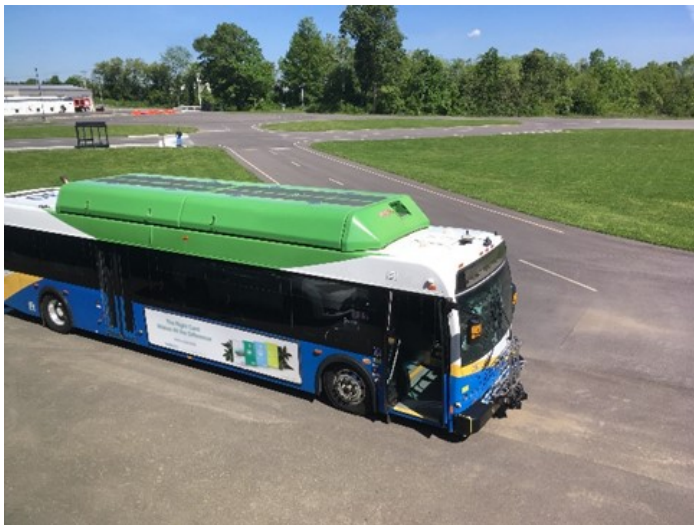
A Pierce Transit bus equipped with the AEB system being tested at the VTTI Smart Road Facility. The front of the bus is equipped with LIDAR sensors, which look like small black boxes installed on the front bumper. Photo courtesy of VTTI.
