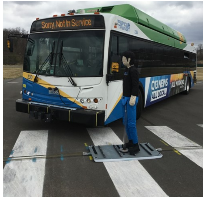
Simulated pedestrian collision avoidance test of Pierce Transit bus equipped with LIDAR detectors on front bumper at VTTI Smart Road test track. Photo courtesy of VTTI.
