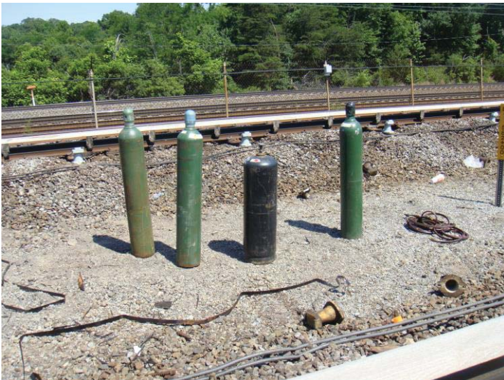
Figure 2 - Freestanding compressed gas cylinders. 3 - Oxygen, 1 - Acetylene
