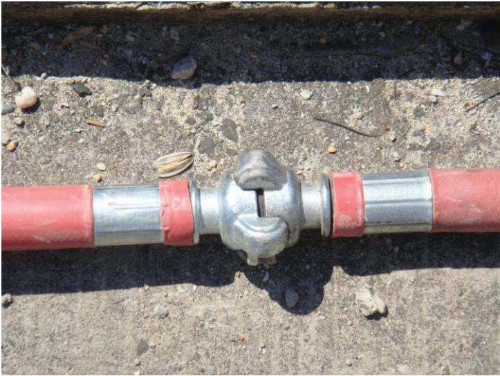
Figure 1 - Chicago air compressor line - no "Whip Check", pins or wire ties
