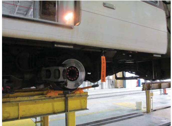
Figure 2: New type plastic manual wheel stops with long handles. The new flag is also placed on the car underframe.
