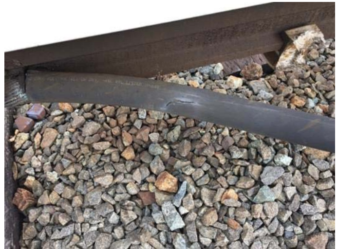
FIGURE 10 - YCR 69 – NICKED PIGTAIL
