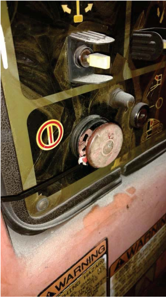
Figure 3 - JLG Lift - E-Stop Button - Tie-Wrap around button
