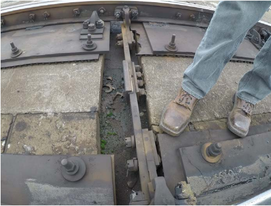
Photo 2: Switch rod number four contacting concrete pad supporting switch nine at C1 360+70.
