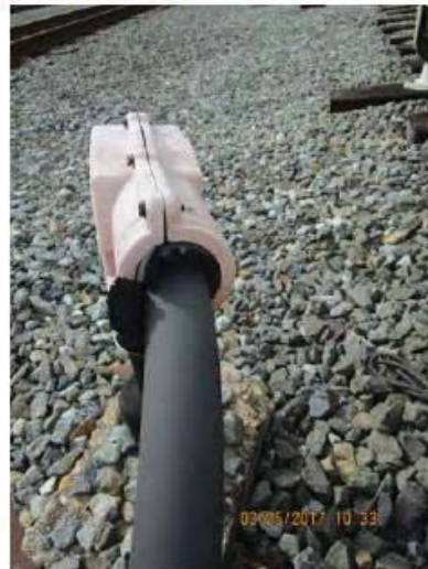
FIGURE 16 - YCR 60 – NEOPRENE SLEEVE COMPROMISED ON ORANGE BOOT
