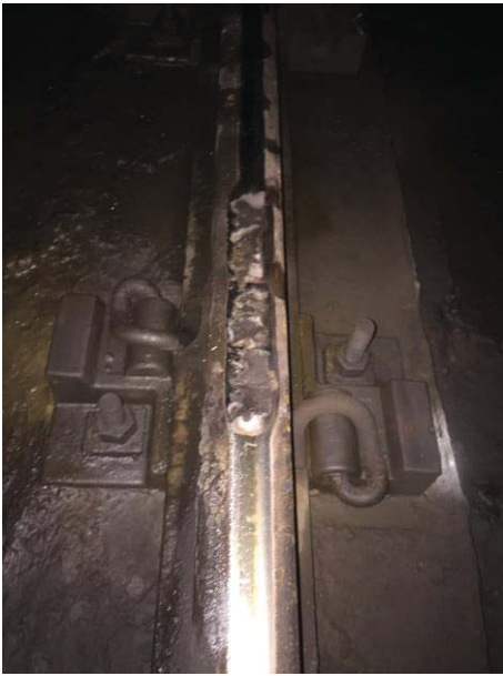
Damaged running surface of rail.
