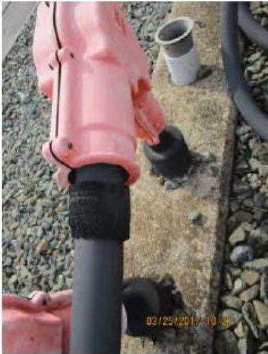
FIGURE 7 - YCR 78 – NEOPRENE SLEEVE COMPROMISED ON ORANGE BOOT
