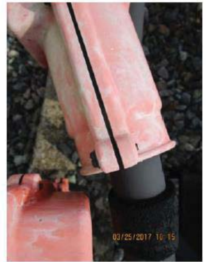
FIGURE 3 - YCR 64 – NEOPRENE SLEEVE COMPROMISED ON ORANGE BOOT
