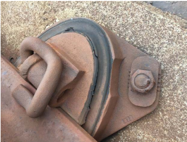
Broken and cracked egg fasteners. 360 degree cracks, not secure to the fastener and allowing rails to float, which threatens track geometry.
