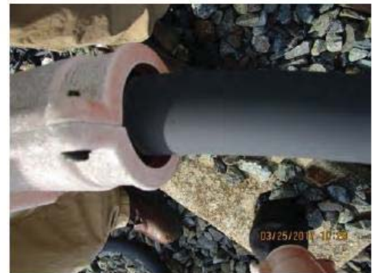
FIGURE 12 - YCR 124 – NEOPRENE SLEEVE COMPROMISED ON ORANGE BOOT
