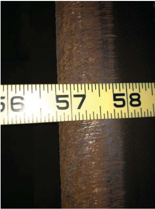
Figure 1: At K1 256+15, 56 ¾ inch static gauge.
