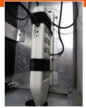
POWER OPTIONS Battery Pack 7-Ah 12 VDC battery; Manual data retrieval Battery Pack w/ Solar Panel
