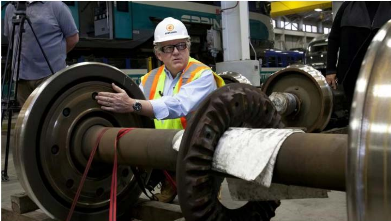
At the Sprinter maintenance facility in Escondido, Bob Young General Manager Operations of Maintenance for Bombardier shows an example of the brake rotor that are prematurely wearing out by as much as 12 months. The brake rotor which has been unbolted from the wheel assembly is the object in the center of the axle. (Nelvin C. Cepeda)
