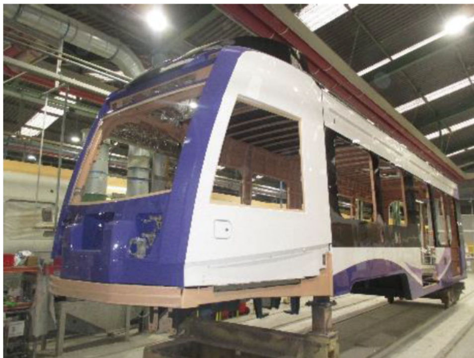
Photo 2: Manufacture of a Purple Line LRV carshell in Beasain, Spain
