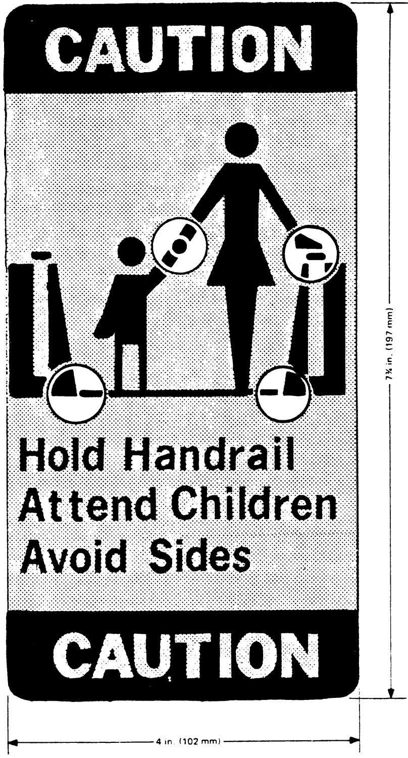
FIGURE 5-1. ESCALATOR CAUTION SIGN
