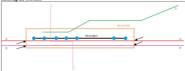
Exhibit 2 shows where in this example the number of riders on-board the transit vehicle needs to be identified. The arrows indicate the location and direction of the on-board load that should be reported.
