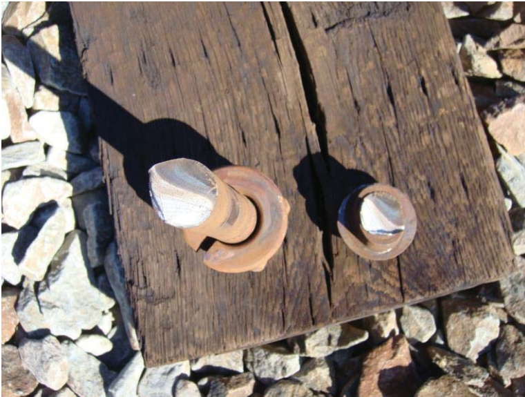
Figure 3 - Broken Bolt from K1 CM604+90
