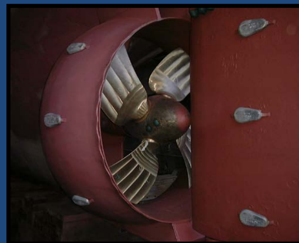
Nozzles Enclosing Propeller to Reduce Friction Losses
