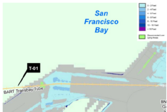
Projected Inundation with 55 inch SLR + 100-yr SWEL
