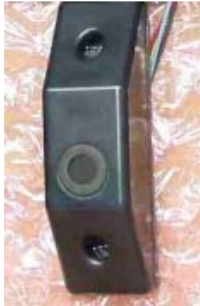
Figure 3-2: Clever Device’s Ultrasonic Sensor 9
