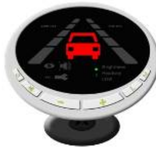
Figure 3-9: Mobileye's DVI Demonstrating FCW 16
