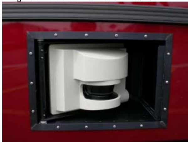
Figure 3-16: SCWS Retractable Laser Scanner 26
