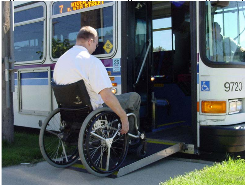
Figure 26 Website Image Showing Wheelchair Loading by Ramp
