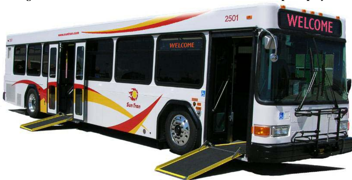
Figure 23 Sun Tran Low-Floor Bus with Front and Rear Ramps Deployed
