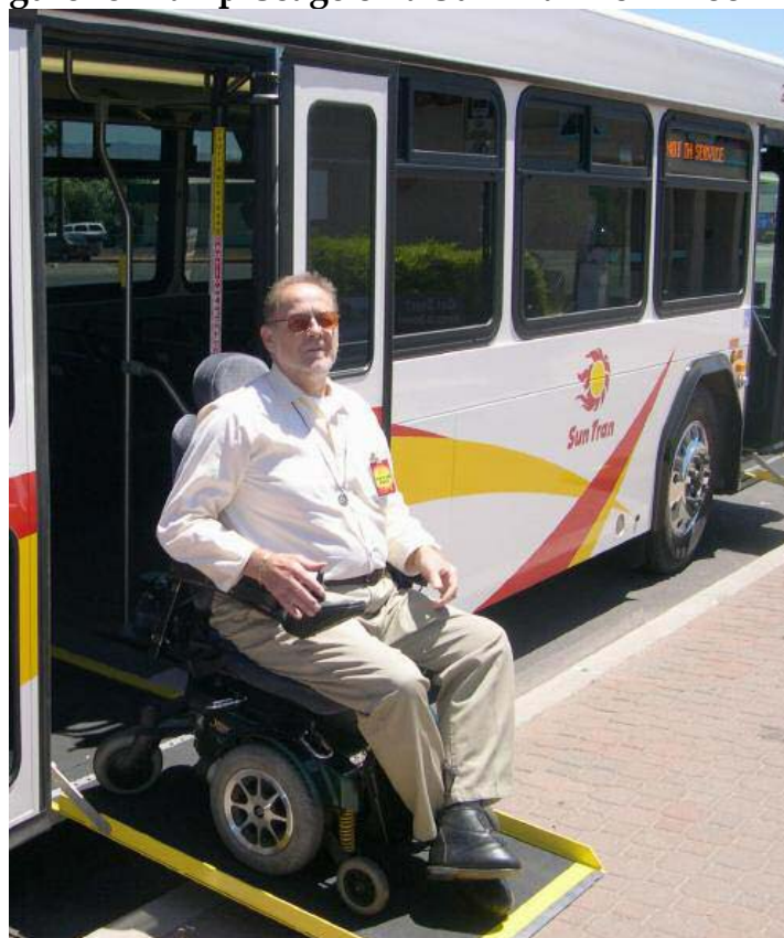
Figure 25 Ramp Usage on a Sun Tran Low-Floor Bus
