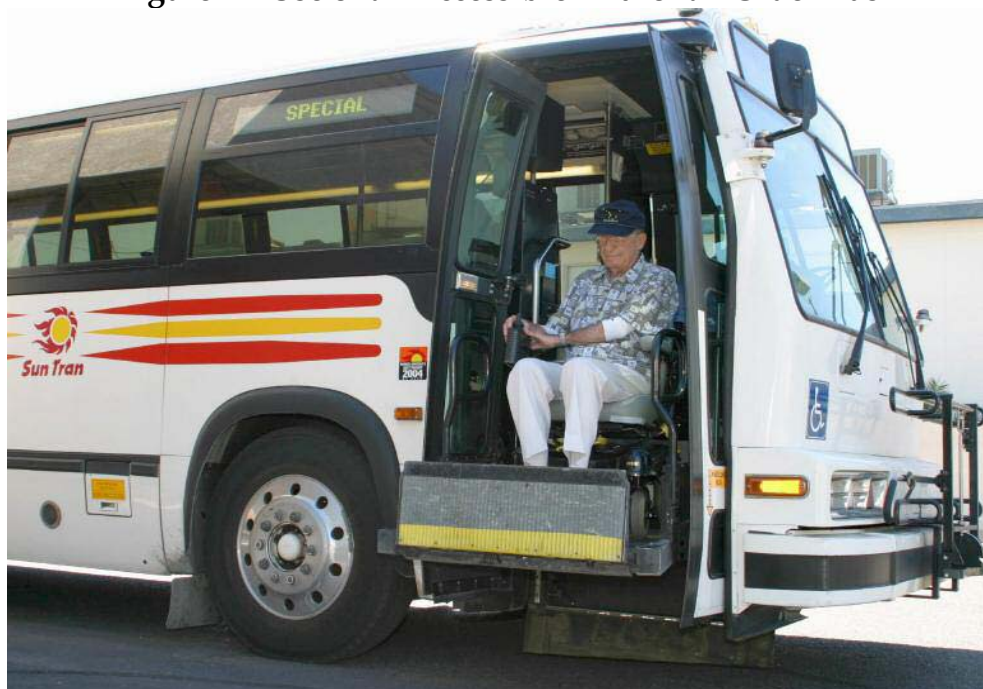
Figure 24 Use of an Accessible Lift for an Older Bus
