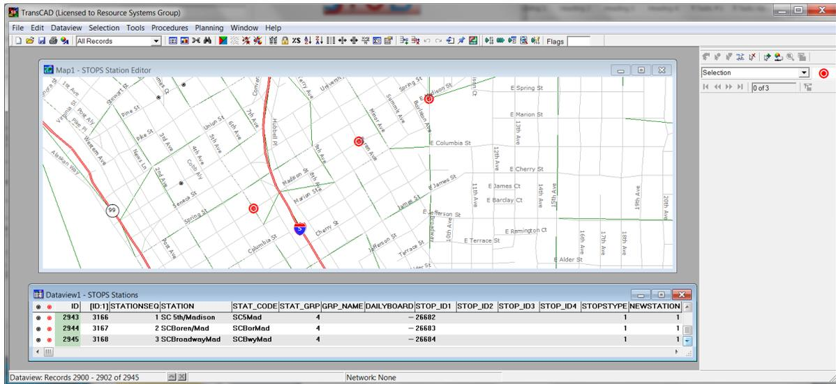
Figure 59. Adding New Stations to Station File
