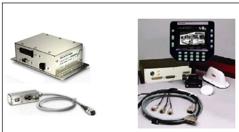
Figure 4-14: Components of APC System
