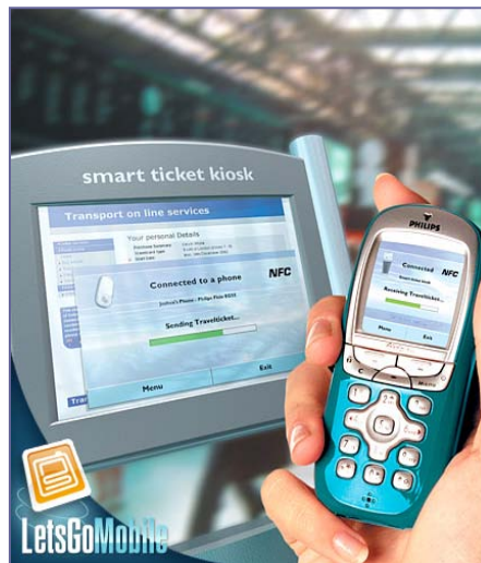
Figure 17: Near-field communications (NFC) enables mobile ticketing
