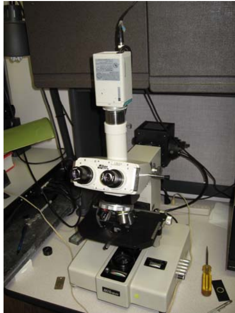
Figure 30 Microscope with test apparatus and cross-polarized light
