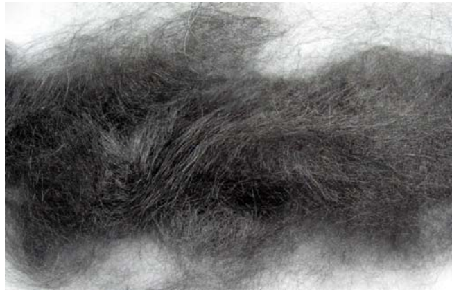
Figure 39 A bundle of carbon fibers (continuous fibers)
