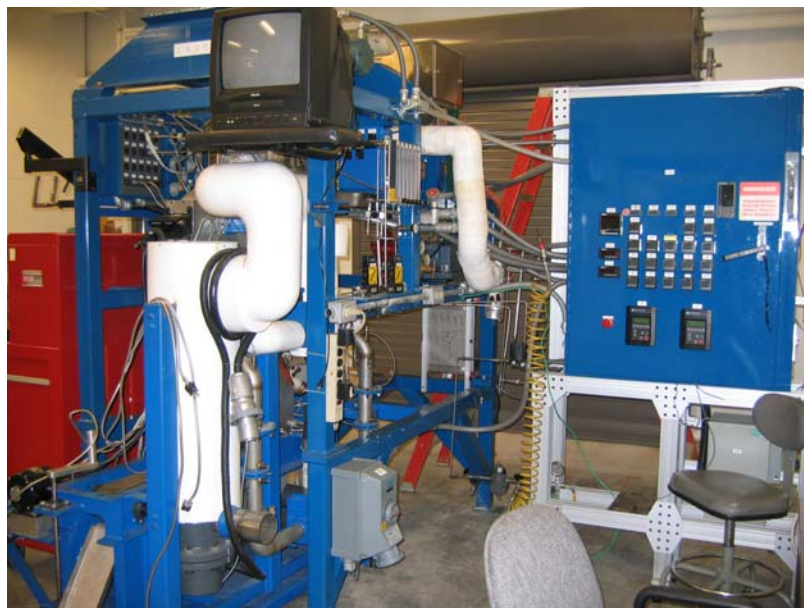
Figure 2 UTISI Spin Lab, a close view of the spin tower, control panel and the fiber collection platform with the secondary gas heater (white duct) in the foreground
