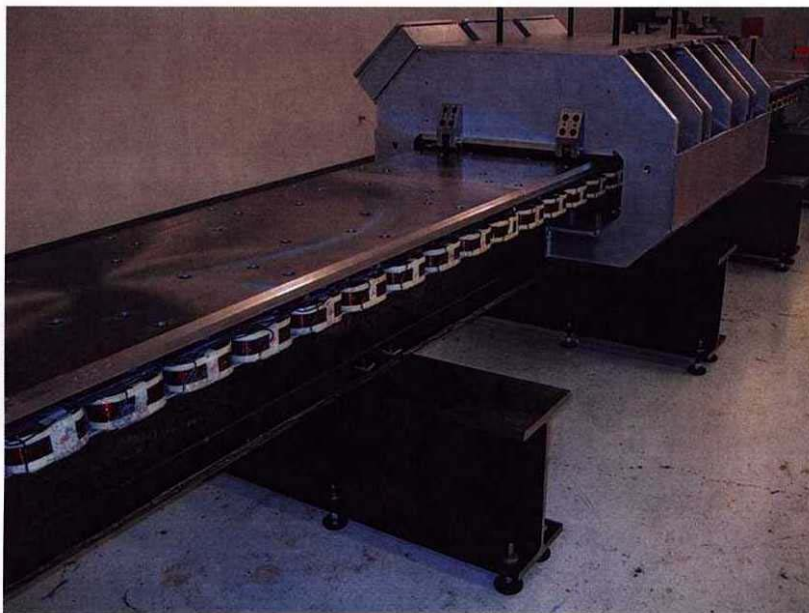
Figure 2. Photograph of the Low Speed Prototype Showing Vehicle, Guideway, and Propulsion Coils
