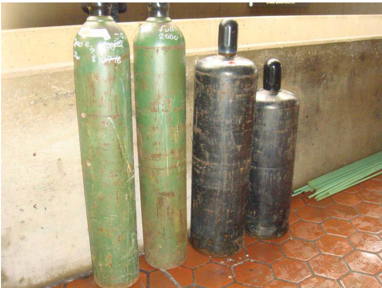
Figure 1 - Un-secured Oxygen CGC alongside Un-secured Acetylene CGC
