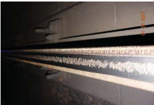
Figure 2: 219+90 low rail spalling
