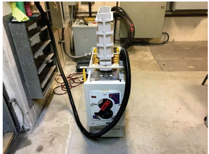
FIGURE 3 – USING TEST CABINET TO TEST OPEN/CLOSE MECHANISM OF CIRCUIT BREAKER
