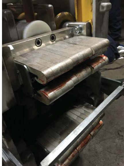
Figure 6 – COPPER BUS STABS OF BREAKER
