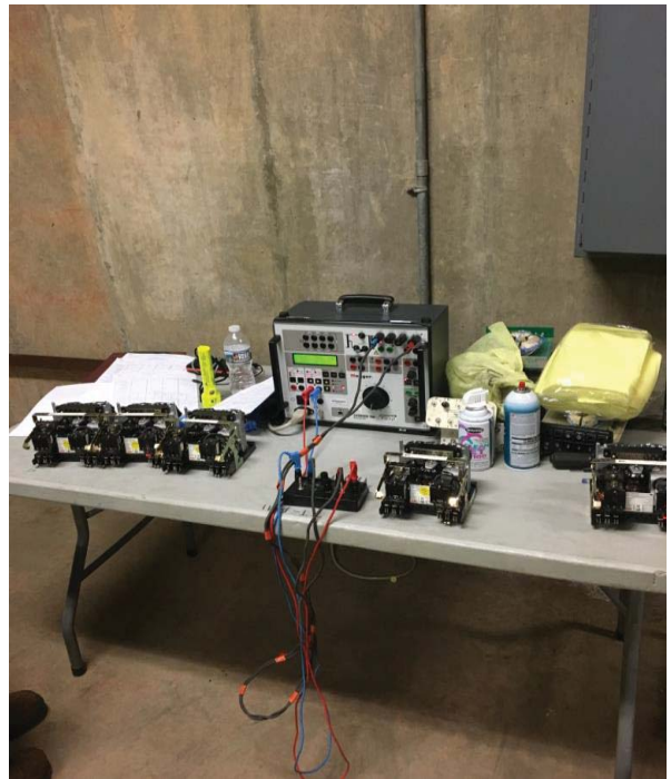
FIGURE 4 - TEST APPARATUS FOR RELAYS
