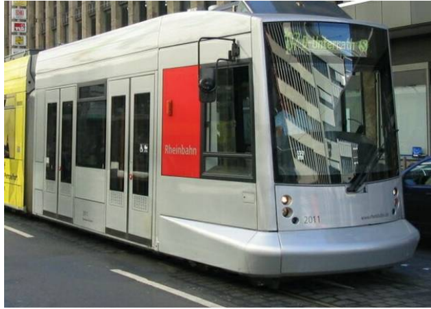
Figure 6. Low bumper profile on the Dusseldorf tram.
