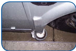
Cleveland BRT bus with guide-wheels for precision docking
