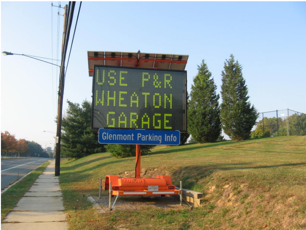
Figure 2-2: Automated Parking Information Signs at Georgia Avenue
