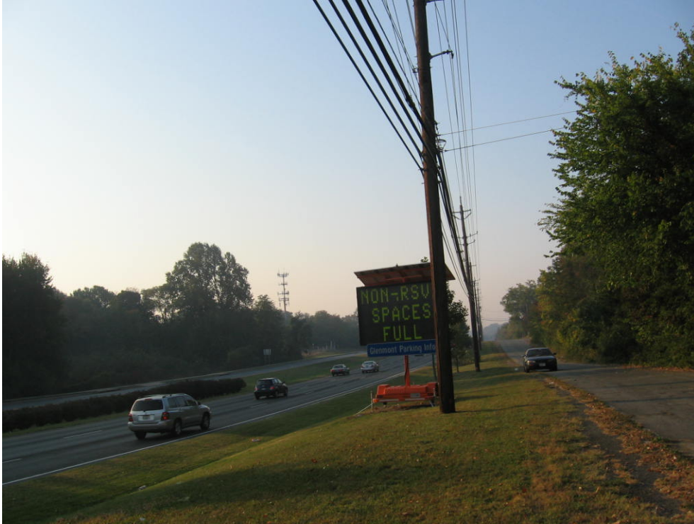
Figure 2-1: Automated Parking Information Signs at Georgia Avenue
