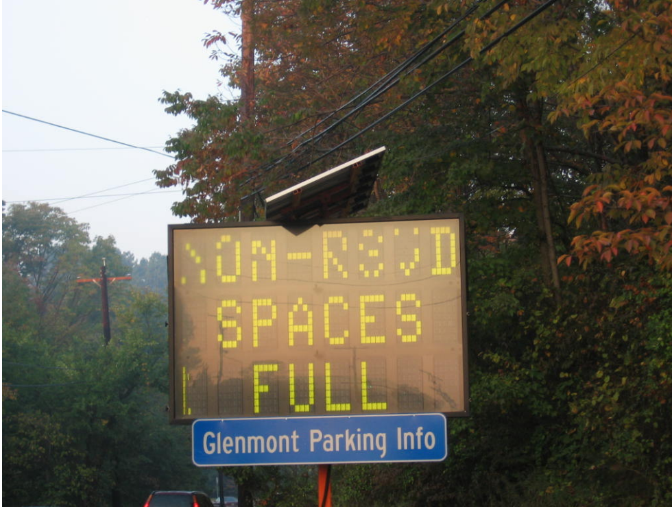
Figure 2-3: Automated Parking Information Signs at Norbeck Road
