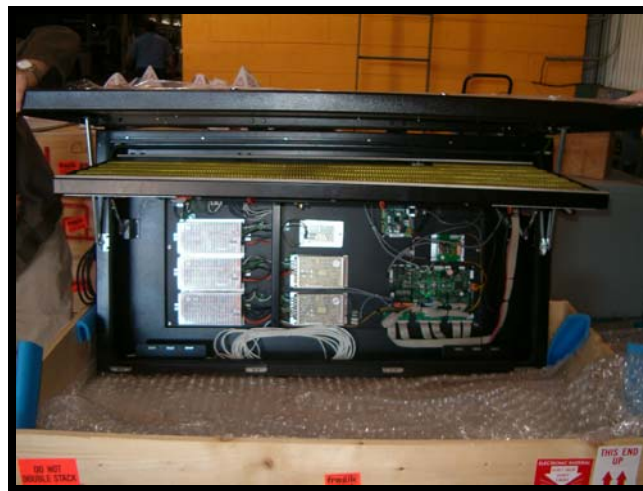
Figure 14. DMS Sign Circuitry
