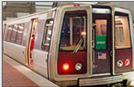
An electric railway that operates local service in exclusive right-of-way. The service is characterized by long trains of six to eight cars or more and by relatively short distances between stops for local service within a city and the immediate suburbs. The Nation's traditional subway systems are classified as heavy rail.
