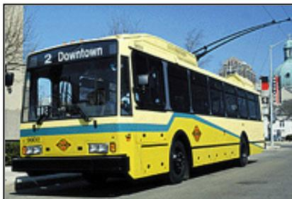
Fixed-route service using rubber tire buses powered by electric current from overhead wires using trolley poles. Service using rubber tire replica trolleys or historic trolleys, powered by an on-board motor are not included in this mode.
