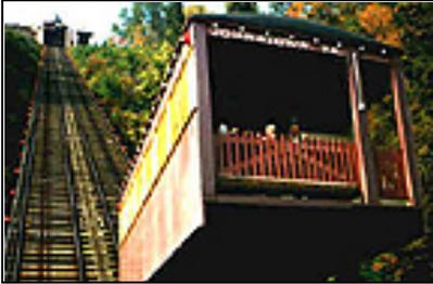
A railway operating on steep slopes and grades with vehicles powered by moving cables.
