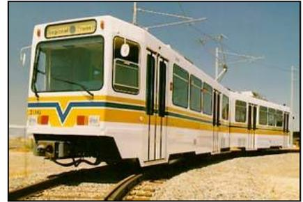
An electric railway that operates local service in mixed traffic with road vehicles, or has grade crossings with roadways. The service is characterized by short trains of one to four cars and by relatively short distances between stops for local service within a city and the immediate suburbs.
