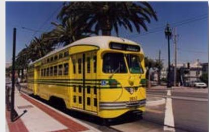
Rail systems operating routes predominantly on streets in mixed-traffic. This service typically operates with single-car trains powered by overhead catenaries and with frequent stops.
