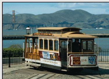
A railway propelled by moving cables located beneath the street. While popular at the turn of the last century, the only surviving system is operated in San Francisco.
