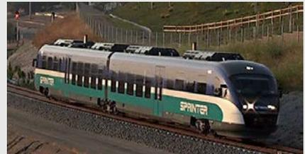
Rail systems primarily operating routes on the National system of railroads, but not operating with the characteristics of commuter rail. This service typically operates light rail-type vehicles as diesel multiple-unit trains (DMU's).
