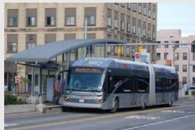
Fixed-route bus systems that operate at least 50% of the service on fixed guideway. These systems also combine passenger stations, traffic signal priority or pre-emption, low-floor vehicles or level-platform boarding, and separate branding of the service. This is often a lower-cost alternative to light rail.
