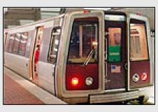
An electric railway that operates local service in exclusive right-of-way. The service is characterized by long trains of six to eight cars or more and by relatively short distances between stops for local service within a city and the immediate suburbs. The Nation's traditional subway systems are classified as heavy rail. Hybrid Rail (YR) Rail - Fixed Guideway
