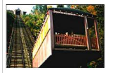
A railway operating on steep slopes and grades with vehicles powered by moving cables.
