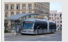
Fixed-route bus systems that operate at least 50% of the service on fixed guideway. These systems also combine passenger stations, traffic signal priority or pre-emption, low-floor vehicles or level-platform boarding, and separate branding of the service. This is often a lower-cost alternative to light rail.
