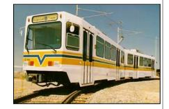
An electric railway that operates local service in mixed traffic with road vehicles, or has grade crossings with roadways. The service is characterized by short trains of one to four cars and by relatively short distances between stops for local service within a city and the immediate suburbs.
