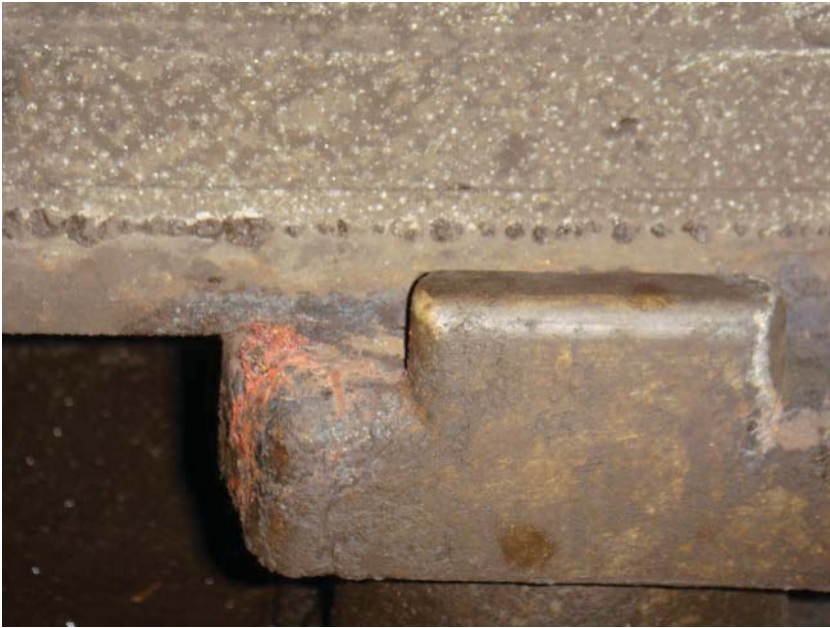
Figure 3 - Insulator at A1 CM 427+30 - appears to be arcing
