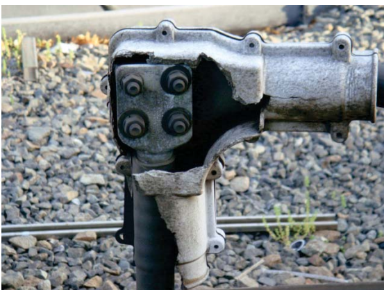
Figure 5 - Cracked Boot - Exposed connection - K1 CM 536+00
