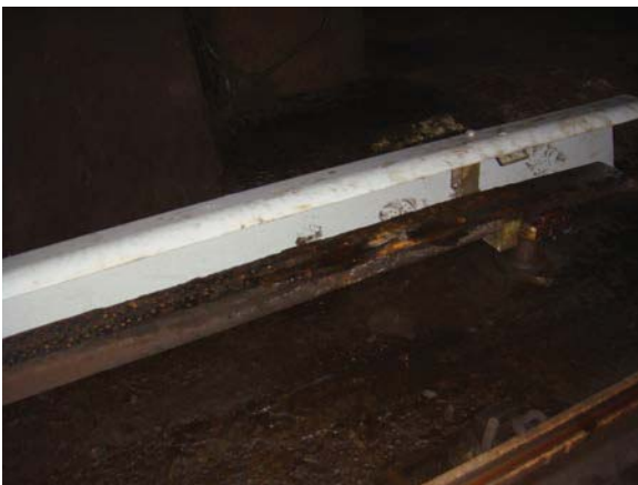
Figure 3 - End approach with sediment and insulator with appearance of charring
