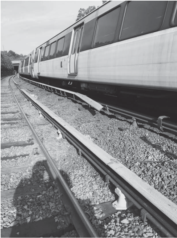
Figure 2 - Hanging Cover Board observed on track #2
