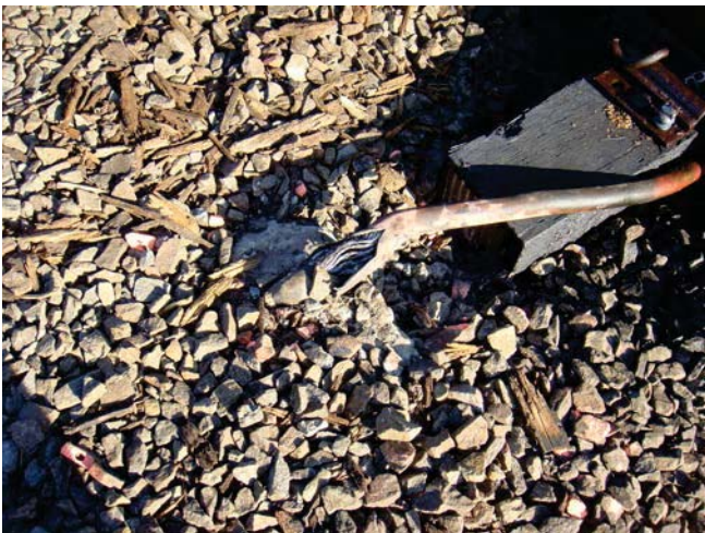
Figure 1 - Damaged 3rd Rail Return Cable
