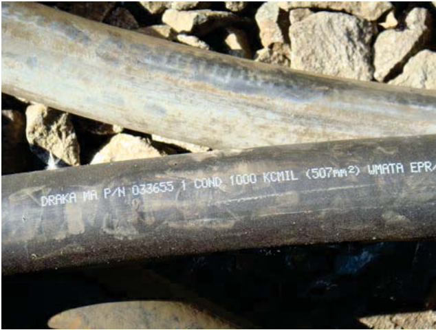
Figure 2 - Cable used to replace expansion joint jumpers -#1
