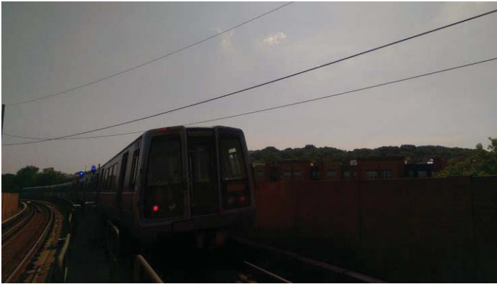
Figure 3 - CM305+00 - low hanging transmission line - (Photo courtesy of WMATA unit #634)
