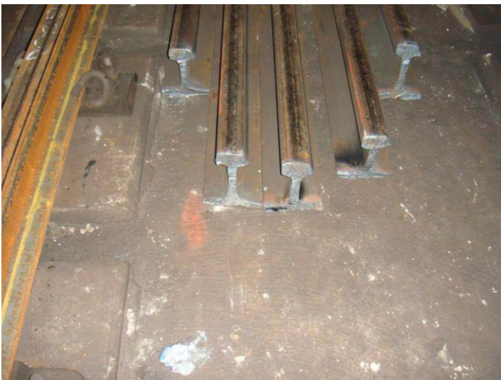
Figure 5 - removed rail - note right side side-wear
