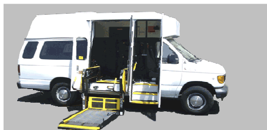
This Braun conversion van is retrofitted with a wheelchair lift.
