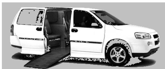
This Braun minivan is retrofitted with a wheelchair ramp.
