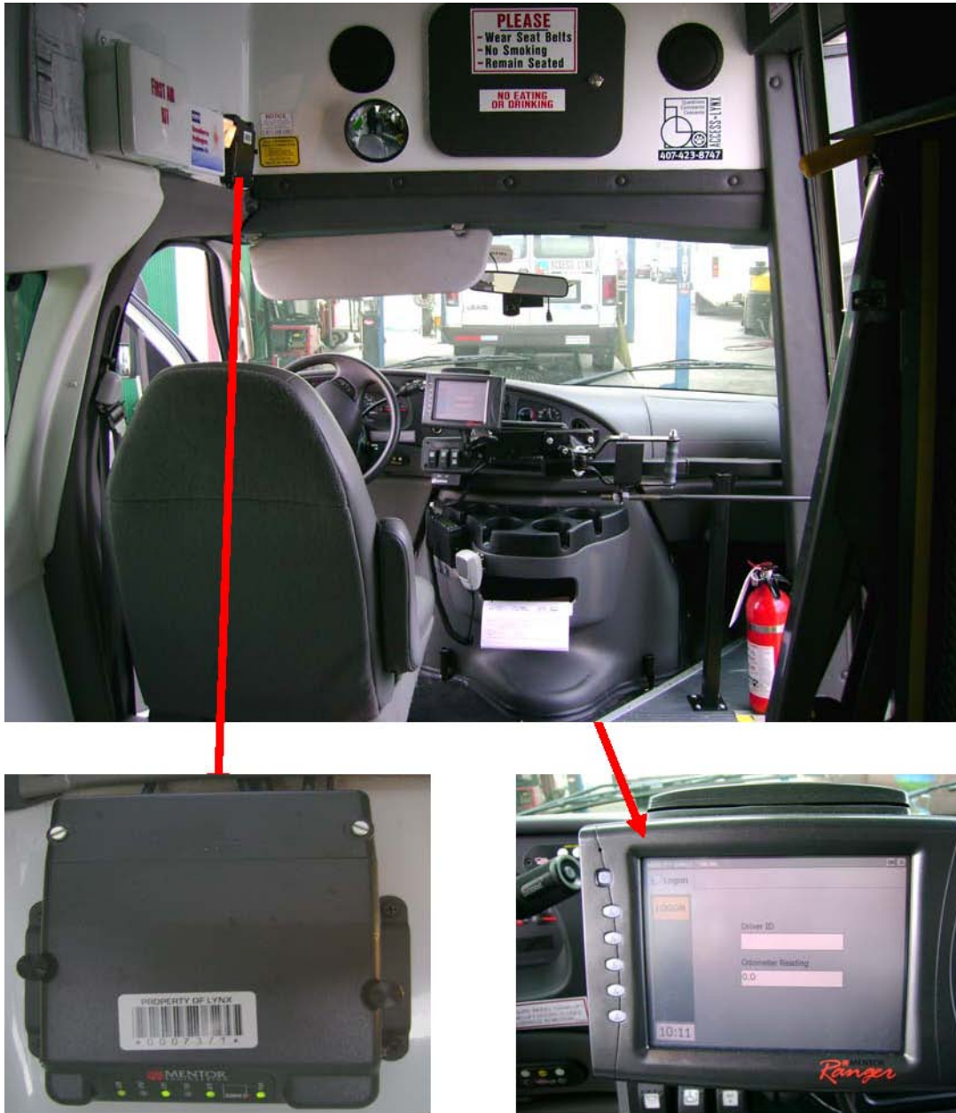
Figure 4: ACCESS LYNX Equipment Layout and Key Components
