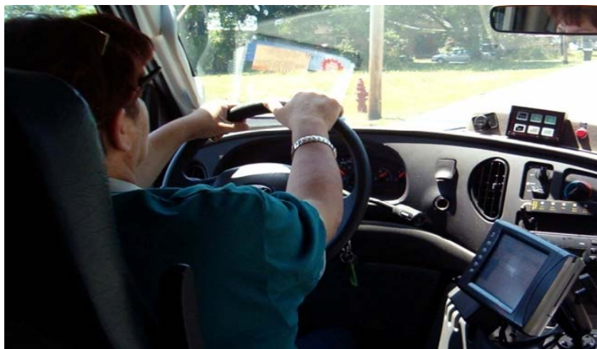
Photograph of the driver's compartment of a Polk County Transit Services' paratransit vehicle with a mobile data terminal (MDT).
