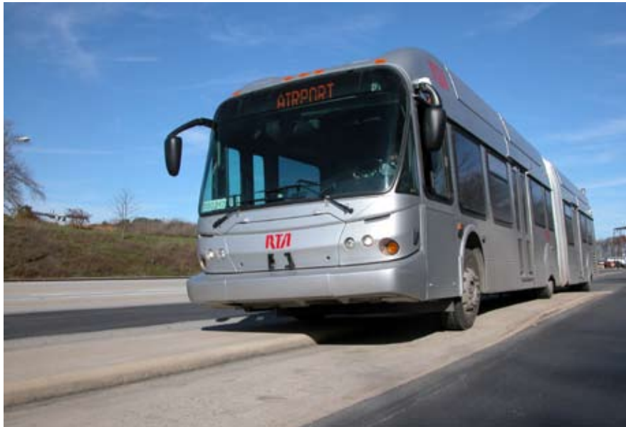
Cleveland RTA BRT bus on the durability track at the Altoona Bus Research and Testing Center (BRTC).
