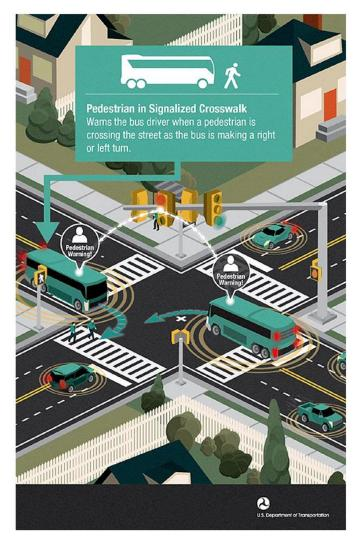
Figure F-I Connected Vehicle V2I pedestrian warning system
