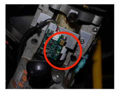
The type, length, and frequency of the auditory warning can be customized. Using standard computer sound files, the warning can be developed by an agency and installed onto the system's ECU, which is housed inside the bus behind the bus operator cabin. The auditory warning can be a verbal message or a sound/tone, can vary in length, and can be set to play only once or multiple times during the turn.
