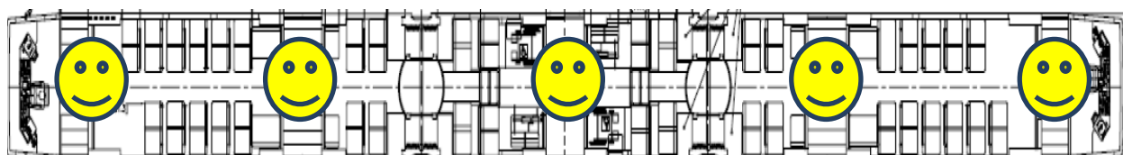
Figure E-3. Location of Human Counters at Each Doorway of an APC-equipped SLRV (Source: DART)
