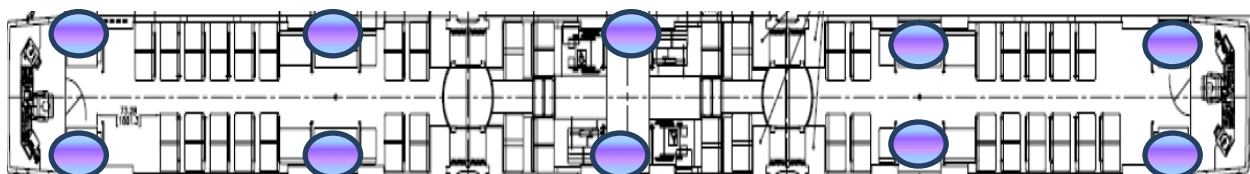
Figure E-4. Location of APC's Equipment at Each Doorway of an APC-equipped SLRV (Source: DART)
