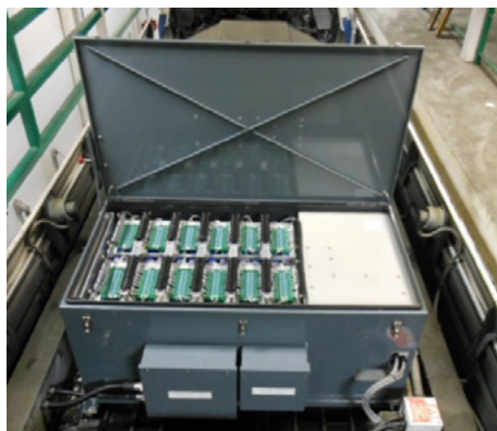
Figure 7-76 Ultracap Energy Storage Installed on TriMet LRV
