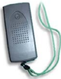
Figure 2-3 RIAS receiver with a neck strap
