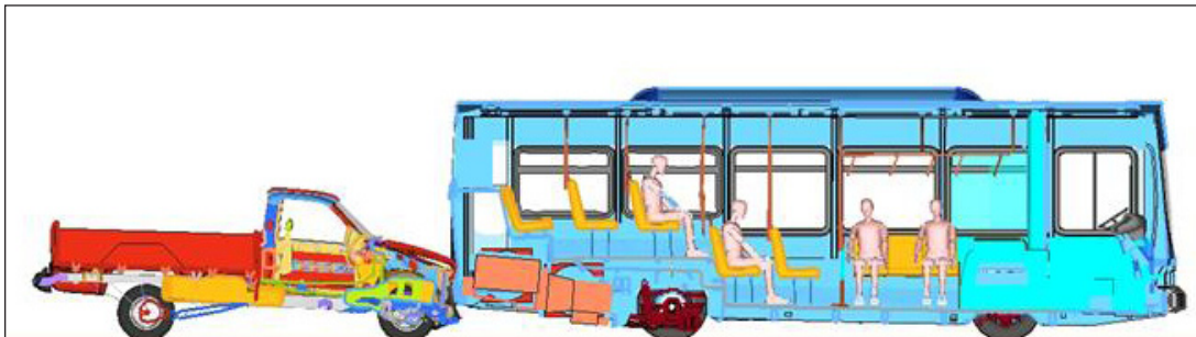
Wichita State University evaluated transit-bus-vehicle compatibility during front- and rear-end simulated collisions.
