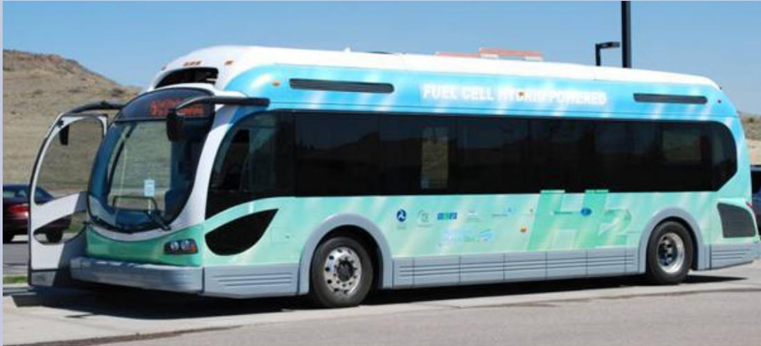
The 35-foot Proterra Inc. hybrid electric fuel cell bus has a lightweight composite body.
