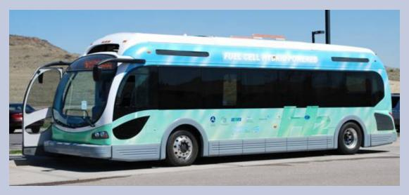
The 35-foot Proterra Inc. hybrid electric fuel cell bus has a lightweight composite body.
