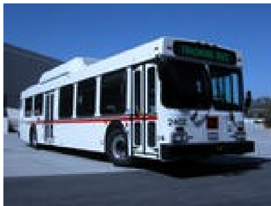
40-Foot ISE-New Flyer Gasoline Hybrid Bus in Long Beach Courtesy ISE Corporation
