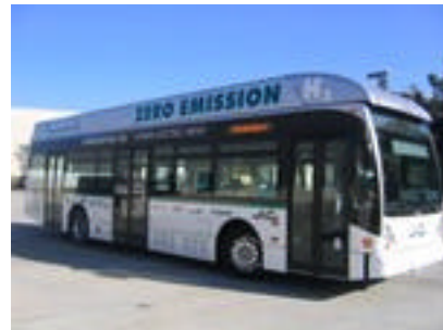
40-Foot Van Hool Fuel Cell Prototype Bus with UTC Fuel Cell System
