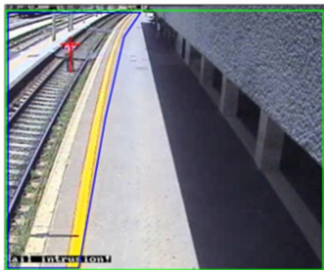
Figure 2-3 Trespasser Detection – Activity on Rail Track at Railroad Station
