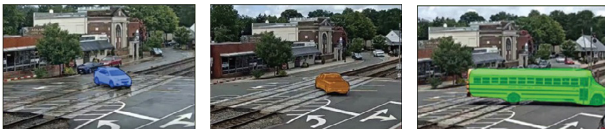
Figure 2-1 Trespassing Vehicle Detection – AI-Based Detecting Algorithm
