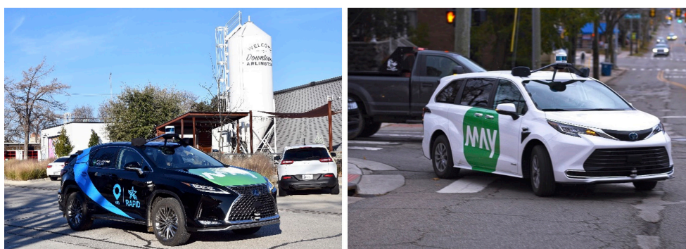
Figure 3-2 Lexus RX450h and Toyota Sienna equipped with ADS from May Mobility Photo Credit: May Mobility
